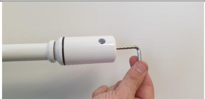
6. Mount the bleaching head by turning clockwise the positioning fixator located on the telescopic arm. By turning the conical fixator located on the straight arm, the telescopic arm is firmly fixed.
