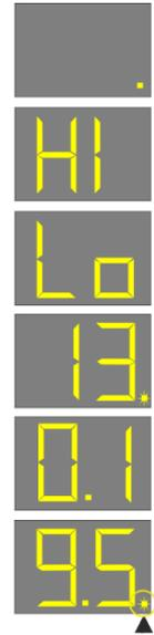
3. The display shows "HI" - a high intensity level. If you want to switch to the "Lo" (Low) intensity mode, press the TIMER / MODE (+ / -) button once. Then the display will show "Lo". Every time before setting the required time, you will be able to select the Hi or Lo intensity level.
