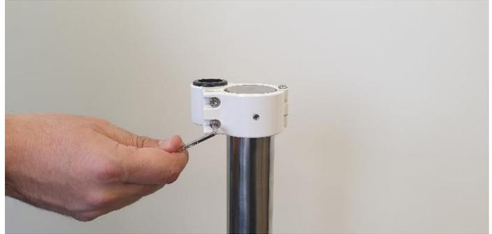
2. Tighten the stop/safety screw with a 3 mm Allen key (included in the package).
