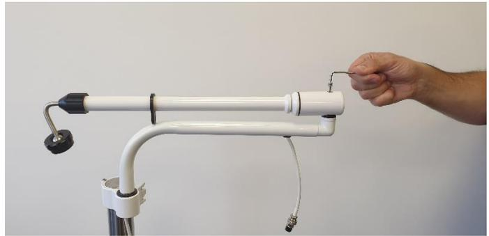
5. Altering the force required to move the straight arm up and down is done by adjusting the screw (located on the back of the central position locking mechanism) with a 5 mm Allen key (included in the package).
