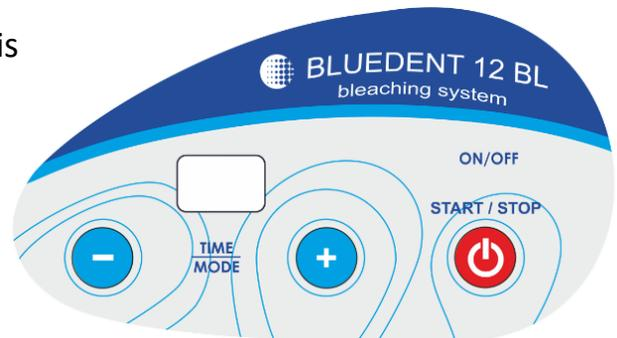
7. To Stop the bleaching device at any time press the START / STOP button. If the device is not manually stopped it will stop after the selected time has elapsed. Note that the fan will continue to work for some time in order to cool down the unit.
